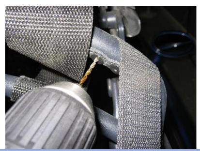
By now, you should have drilled out 10 total rivets. Do not touch the two straps that go between bow #1 and #4. Those straps will not be removed.
