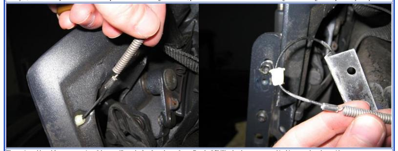
The tension cable and front-most portion of the top will now be free from the top frame. Bag the 8 Phillips-head screws removed in this step and set them aside.
