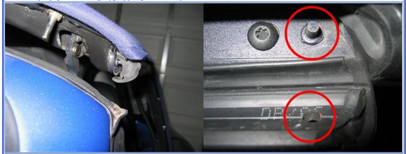
Once all 4 seals are in place, close and latch the top. Check the seals visually to make sure there are no gaps. If there are, open the top back up and realign the seal.
