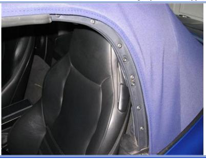
Step 27: Attach the seals to the seal frames.
