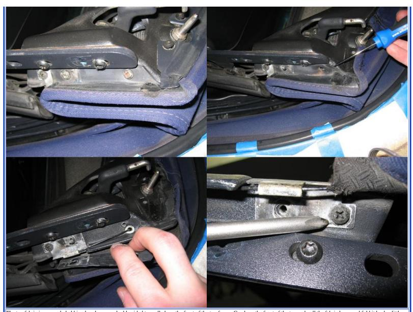
The top fabric is now only held in place by some double-sided tape all along the front of the top frame. Go along the front of the top and pull the fabric loose and fold it back a little. This will expose the locking mechanism in the front of the top frame, as well the mounting for the tension cables.
