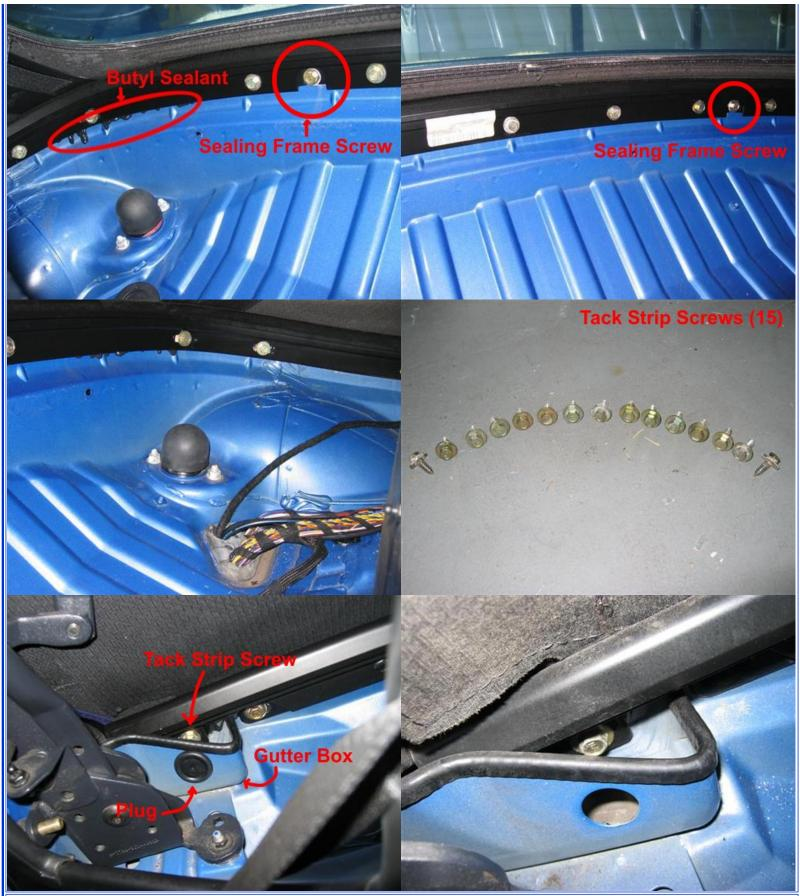
With all the screws removed, you will notice that the tack strip doesn't move freely. This is because it is being held in place by butyl rubber sealant along the outside. Don't worry about this for the time being, as the tack strip doesn't come out until the end of disassembly. Bag all the screws and set them aside.
