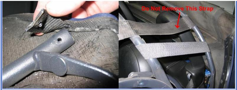
The next rivets are located on on bow #4, and are holding the wide strap to the bow. There are 2 per side with one being on the front of the bow and one in the rear on each side. Drill all 4 out.
