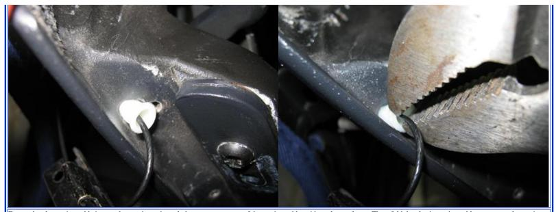
Ensure that the tension cable is routed properly, and attach the rear-most screw of the tension cable guide to the top frame. Then, fold the plastic tension cable cover over the tension cable, and screw it into place with two more Phillips-head screws. This may be difficult on the second side, as the canvas is very tight when new.
